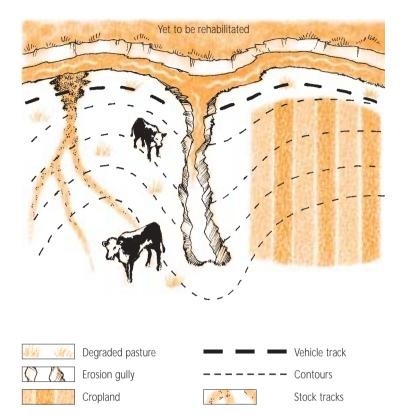
A degraded catchment and riparian land. Significant sediment and nutrient is derived from degraded pasture, poor crop management, unlimited stock access and gully erosion.
