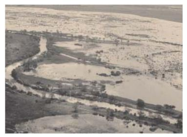
Perched channels occur where the stream bed is higher than surrounding land and is separated by a high bank. An avulsion at this point could cause significant flooding of low lying land below the level of the stream bed, Latrobe River, Victoria. Photo by Chris Gippel.
